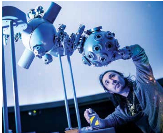
Adam Thung '16 inspects the swing of the lamp shutters during routine maintenance of the ZKP3 optical mechanical.
